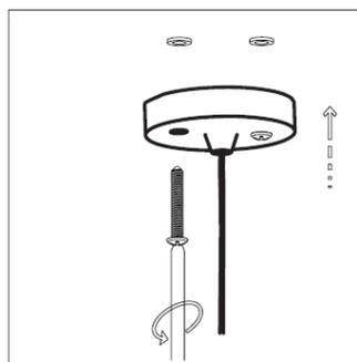
Attach the hangers to the luminaire. The safety lock must be closed, otherwise the luminaire might fall down.
