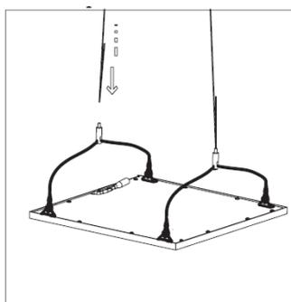
Align the luminaire in the desired height and horizontally.
