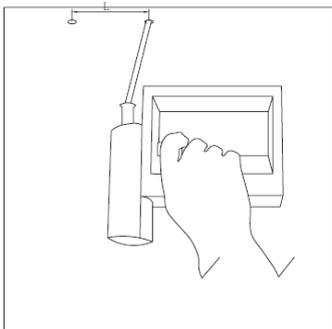
Ceiling thickness must be min. 50 mm, else the luminaire might fall down
